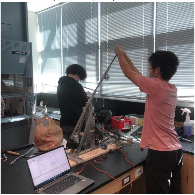
What I was unable to model in inventor was the weights, wires, and vex cortex which can be seen in on the catapult. The cortex contains the necessary code to run the catapult and weights provide the force that launches the projectile. The code can be seen on the laptop.
